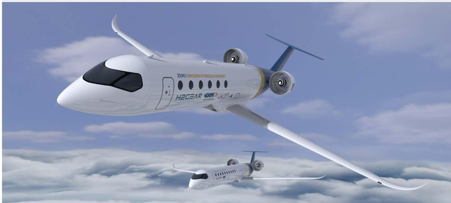
Liquid hydrogen fuel cell commuter-class aircraft concept
